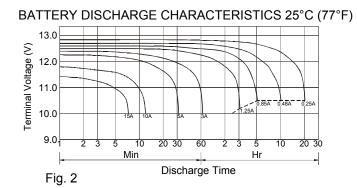
For example, a 5 Ah battery will discharge to 10.5 volts in 30 minutes at a current draw of 5 amps — not a full hour, see Fig. 1. This is asuming constant discharge current, however, and if the battery were allowed to rest the voltage would soon rise sufficiently to allow a 0.5 amp load to run for almost five more hours. See Fig. 2 for voltage vs. discharge time for various discharge currents.
