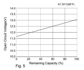
Remaining internal battery capacity can be approximately determined by turning the unit off for at least 24 hours and measuring the voltage at the GND and AUX terminals. Refer to Fig. 5. For example, a measured voltage of 12.4 volts would indicate 50% remaining capacity or 2.5 Ah.
