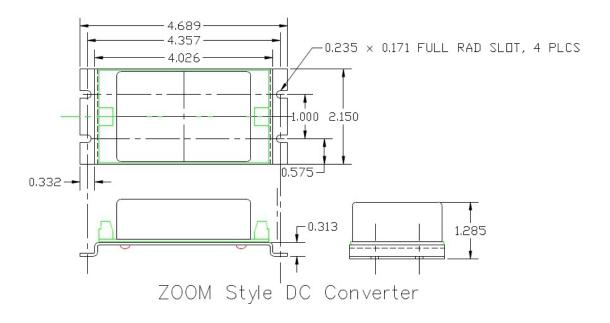
Figure 4. Dimensioned drawing
